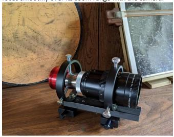
I already had an old pair of mounting rings for the lens, but I needed to jimmy up a mounting bracket for the lens rings to also carry the 60mm guidescope like the 80mm refractor. Had a couple of metal mounting brackets that I thought I could use, but the weren't wide enough so I utilized an old wooden mounting bracket that I also had in the goodie box. While not perfect, it will work until I get something to replace it. Here's a couple of pics showing the installation:
